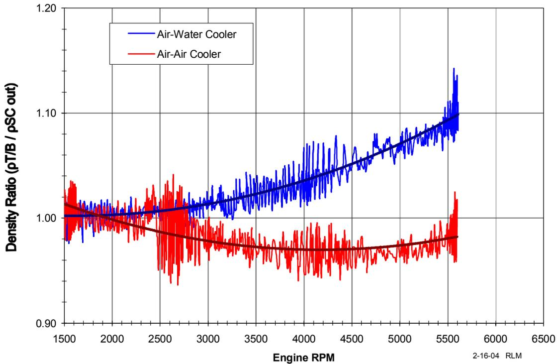
**Figure 6 – Density Ratio performance for air-to-water and comparison “2-core” air-to-air charge cooler systems. 5.0 L Mustang engine dynamometer test. Air-to-water results: 342.1HP at 5400 RPM; air-to-air results: 312.6HP at 5200 RPM (Corrected HP).**
