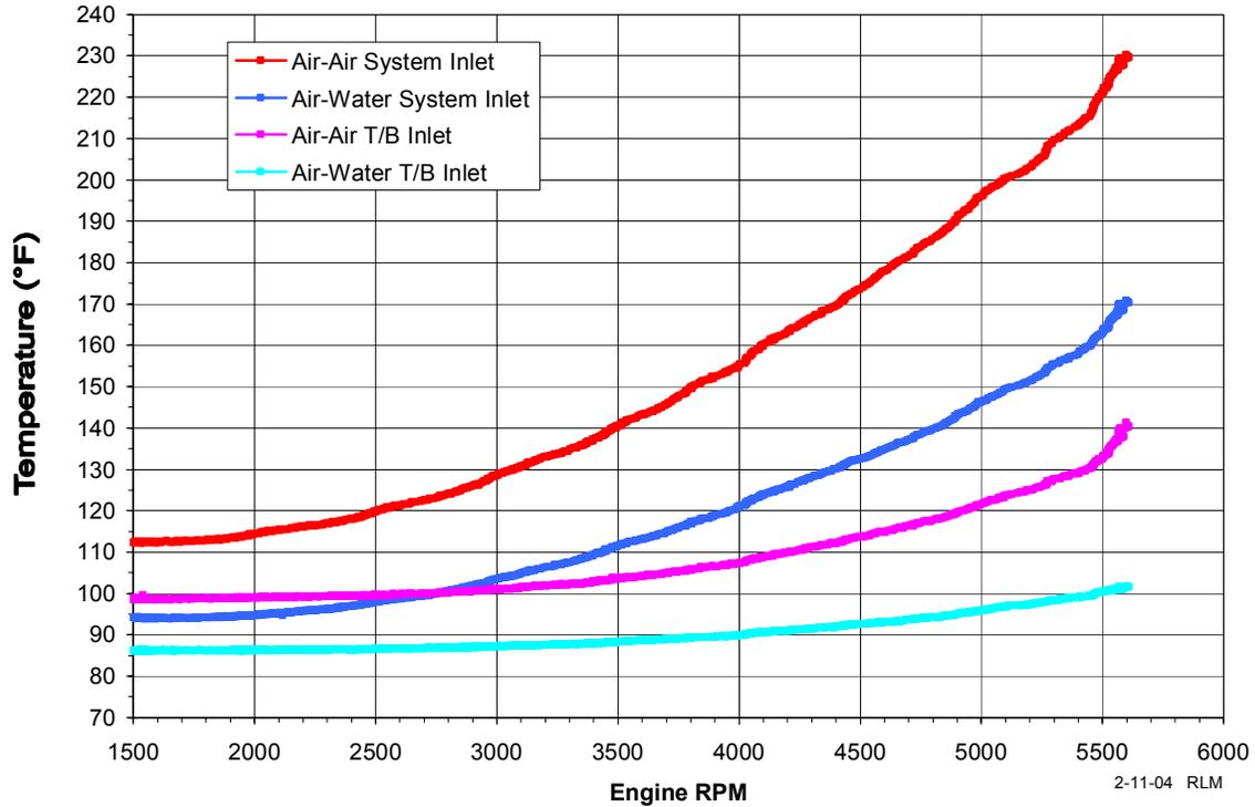
**Figure 5 – Engine Dynamometer Testing – Inlet and discharge temperatures of charge cooler systems. Red + pink is “2-core” air-to-air data; blue + light blue is air-water. Averaged data from same test runs as Figure 4. 5.0L Mustang (1986-1993 M/Y) engine. Ø36” ducted fan used for cooling air supply; tests conducted after warm-up and thermal stabilization of system components.**
