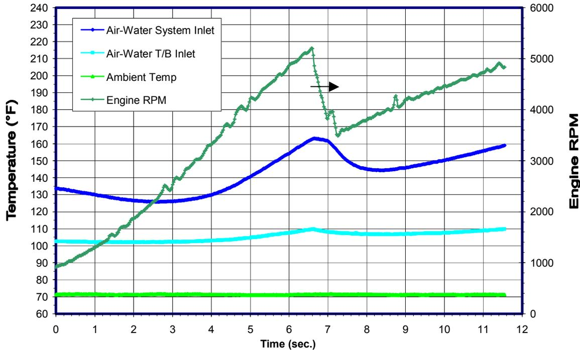
**Figure 9 – WOT Acceleration Road Test – Vortech V1S supercharger with air-to-water charge cooler system. 1991 Mustang 5.0L. Tests conducted after 15 minute (min.) warm-up drive.**
