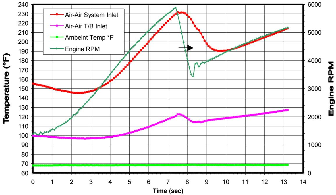
**Figure 8 – WOT Acceleration Road Test – competing supercharger with “2-core” air-to-air charge cooler system. 1991 Mustang 5.0L. Tests conducted after 15 minute (min.) warm-up drive.**
